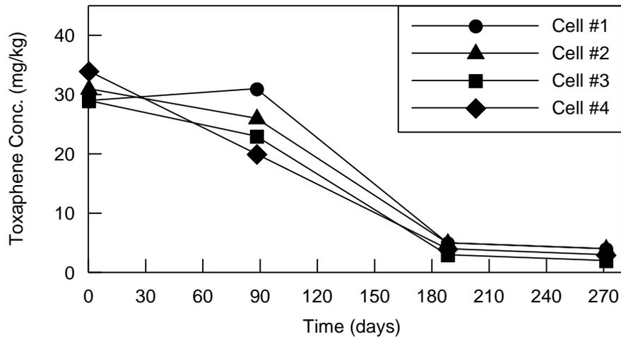
**FIGURE 2. Toxaphene removal in field-scale anaerobic cells at the GRIC site.**
